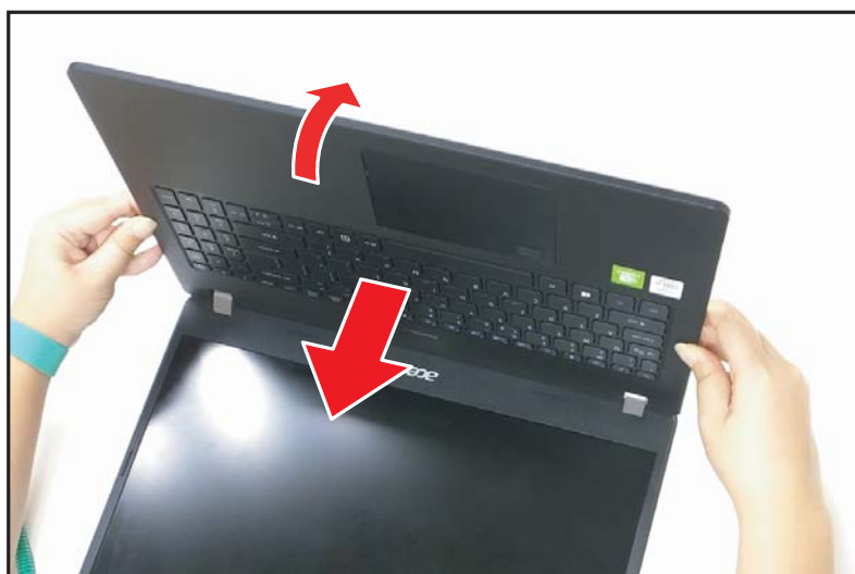
Figure 1-32. LCD Module Removal
