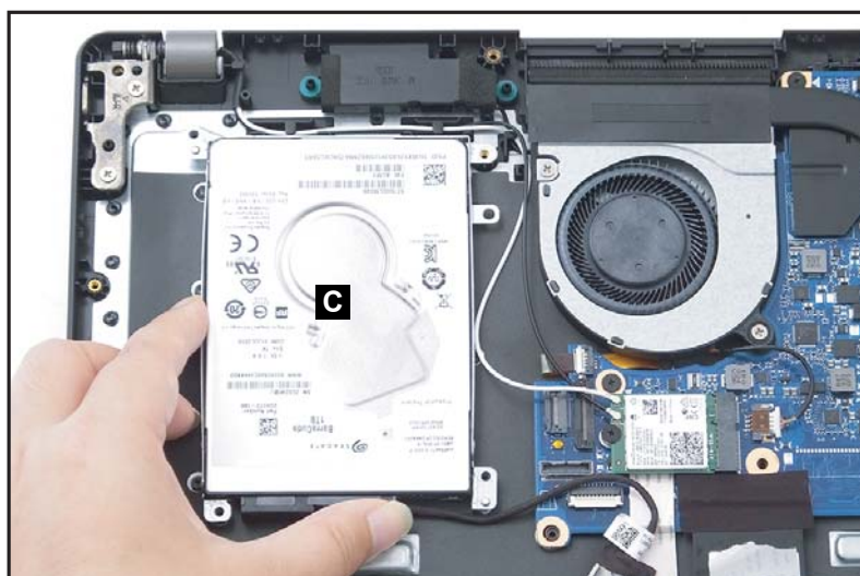
Figure 1-21. HDD Module Removal
